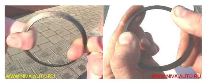
The spring washer must not be oval or distorted in any way:
