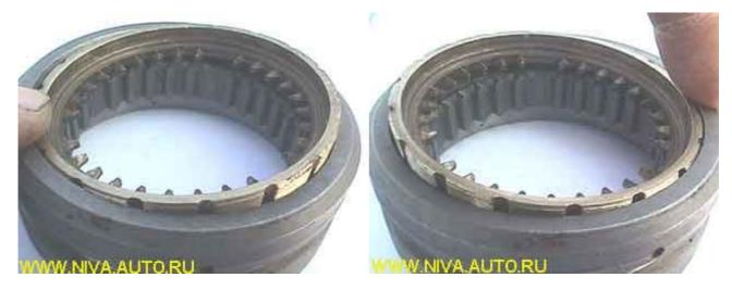
A normal synchronizer baulk ring shouldn't act strongly (below on the right an obviously bad synchronizer) and to be sunk in the sleeve more than  $0.5\ mm$  (at the upper right). The left picture shows a normal synchronizer baulk ring:
