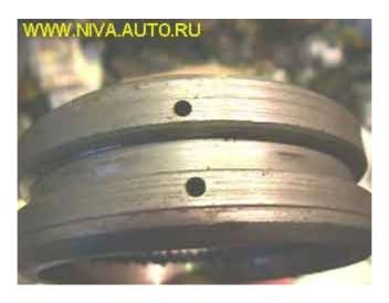
Some defective sleeves are shown below. On the left upper picture one channel is missing, on the right upper picture the channel is obviously displaced to the middle, and the bottom pictures show a badly chamfered sleeve:
