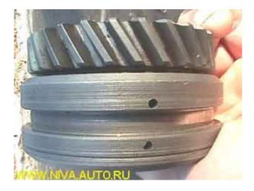
The lubrication channels on the faces of the synchronizer sleeves and gears must not be clogged:
