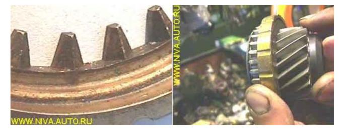
Place the synchronizer baulk ring in its respective sleeve. It should not have any significant ovality:
