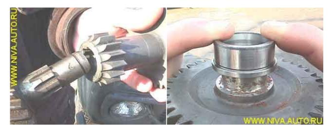
The main shaft: To check the shaft's diameter all gears, bushings, hubs, sleeves, bushes and bearings must be installed on it, on a new shaft all parts should go in with a small tightness. To check the splined end we must insert the rear flange and turn the shaft and flange in opposite directions and look for absence of play between both parts:
