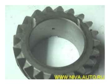
If it's necessary to buy assembled gear/baulk ring sets, check for absence of jamming between the baulk ring and the gear's straight teeth. Also check that the synchronizer spring sits squarely against the persistent ring. The synchronizer baulk ring must travel parallel all along the way, if it doesn't either the persistent ring is warped or the synchronizer's spring is incorrectly installed:
