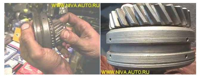
The gear should go on tight, but must enter and exit the sleeve easily without jamming. On the left picture it can be seen that the gear has jammed on the sleeve and can't return to the original position (right picture):
