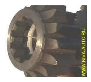
Check the condition of the gear cluster splines. For this purpose the cluster is installed in the rear end of the countershaft (left picture). Also check the landing of the front countershaft bearing inner race (right picture), it shouldn't go in by the hand's force, only with the aid of a hammer:
