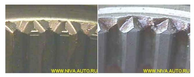
Each sleeve should have 8 lubrication channels. Some channels may appear to have a small displacement relative to each other but this should not be taken as a sign of defects:
