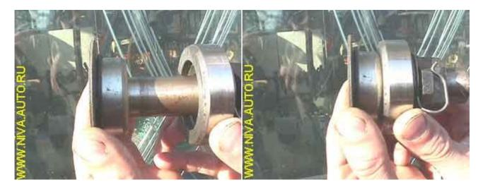
Check the bearing bores in the gearbox **rear cover**. The bearings should go in squarely with effort. The picture shows how the bearing is installed using a hammer wooden handle:
