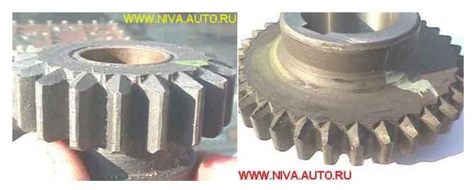
The gear cluster teeth and splines should be symmetrical and free of any damage:
