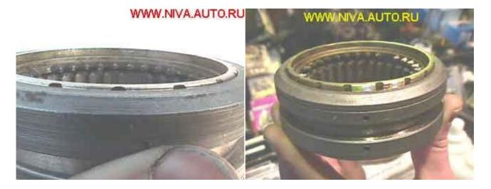
All of the gear straight teeth faces must look precisely equal. The tooth faces must all be symmetrical (see left picture). Shifting to any gear with asymmetrically sharpened teeth (right photo) will prove troublesome:
