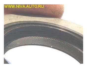
When checking the **release bearing yoke** pay attention to the color and manufacturing quality. The original yoke it's a dark grey color, its spring is kept in place by two small copper rivets. The factory-installed rivets have semi-circular heads. See that the release bearing spring clip holds the yoke snugly:
