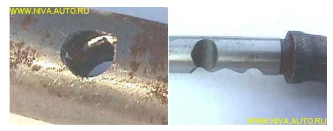
The countershaft should not have any chipped or broken teeth. The ends should have precisely cut threads. Note that the 4-speed gearbox countershaft has an unthreaded rear end (left picture):
