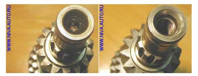
**The reverse gears** should have equal, symmetrical and chip-free teeth. Check the condition of the reverse idler gear brass insert:
