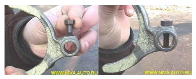
Insert the forks on the sleeves. They should move easily in circles:
