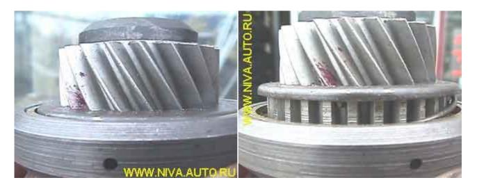
The  $4^{th}$ -speed gear is machined on the input shaft, but it's checked the same way as all others. The picture shows a  $4^{th}$ -speed gear with damaged straight teeth. This condition can't be seen in the picture, but note how the sleeve has jammed on the gear straight teeth and can't come back to its original position under the synchronizer spring action:
