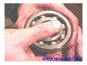
All bearings must be checked to ensure both races rotate relative to each other easily. The needle bearing plastic separator must be free of cracks.
